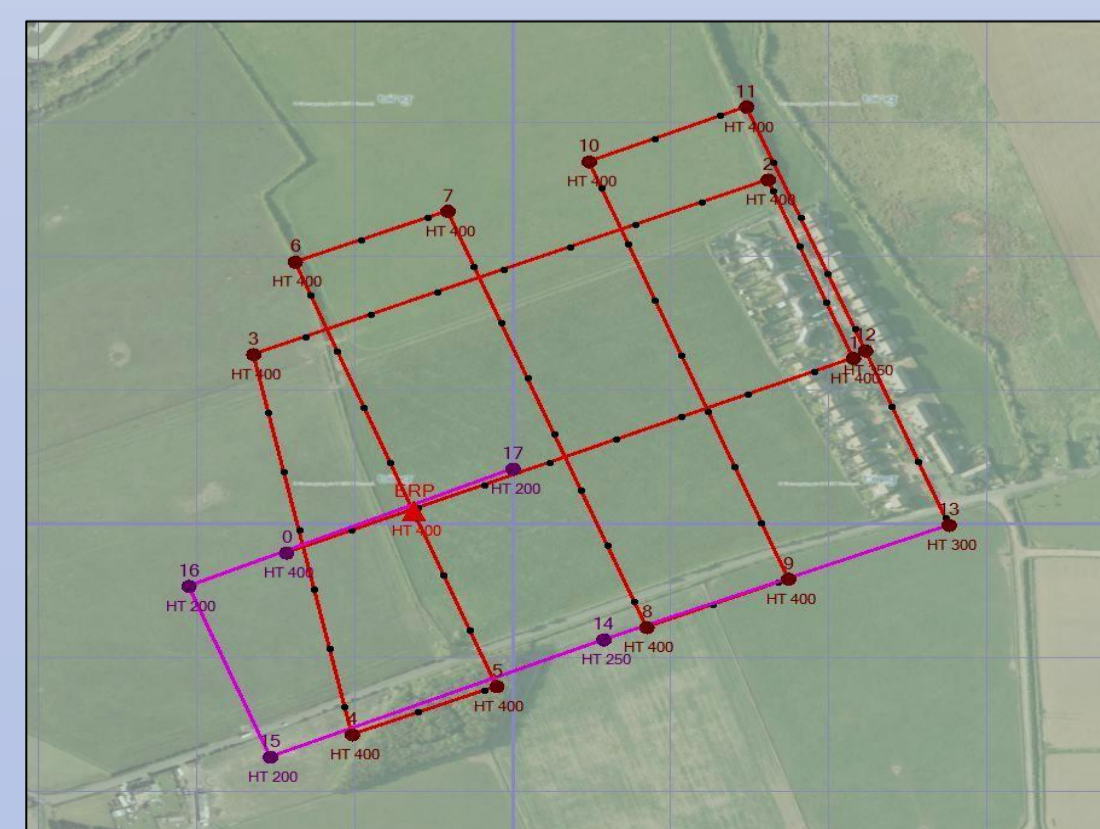
Fig.5: Flight Planning in 'SkyCircuitsPlan' software.
